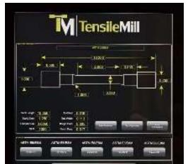
The Tensile Software also makes adding and adjusting specimen sizes extremely easy with the use of our touch screen interface. This is possible for both flat and round specimens. The following video shows this best: <u>https://youtu.be/Nwwo6CJE3XI</u> Irregular or complex specimen sizes can be prepared with the upgraded CNC software.
