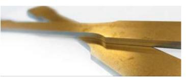
of their raw materials which are often in bulk forms such as sheets or rods. Accurate tensile testing results are highly dependent on the preparation of a tensile sample of the raw material that is of the highest quality.
